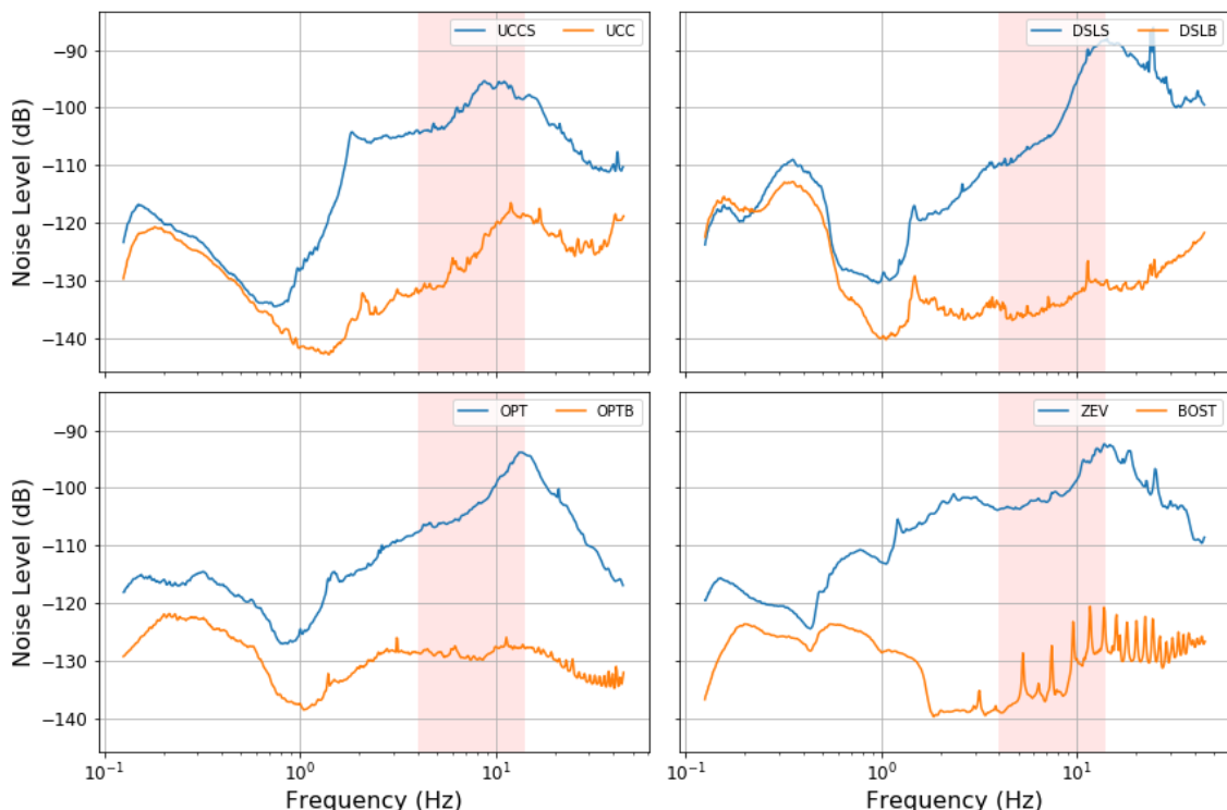
Figure 25: Seismic noise levels difference as a function of the frequency between co-located seismic stations but installed at different depths (blue: surface station and orange: borehole). The red area represents the 4-14 Hz frequency band used for the noise map computations in the previous chapter. UCC = Ukkel-Uccle; OPT = Opitter; OST = Oostende; DSL = Dessel. The noise level in dB units are (m/s^2)^2 / Hz .
